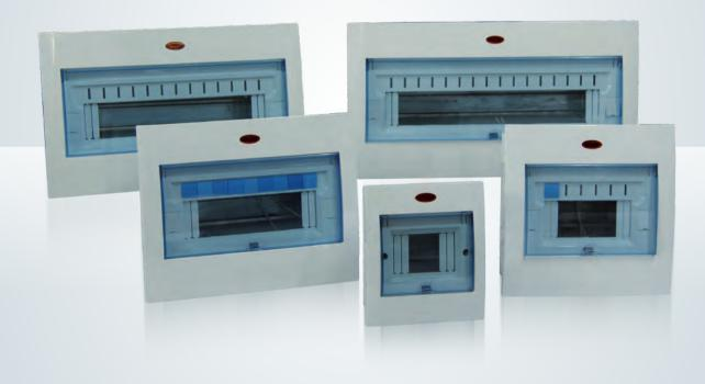
SH series of luxury lighting box is divided into two kinds, Concealed mounted type and Open mounted type. It is with plastic panel and iron bottom. Two terminals (ground connection and zero connection) in the box are easy for the user wiring and routing. This product is applicable to the modular terminal circuit with AC of 50HZ, rated voltages of 220V and 380V.
